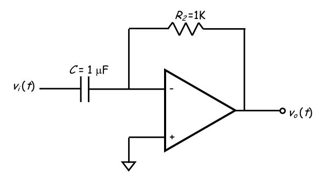
Determine the largest possible value of signal frequency  $\omega$  that would **not** result in a distorted output signal (due to slew-rate limiting).
